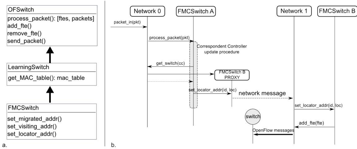
Fig. 3. a. FMC controller object model: the basic OFSwitch class is extended to introduce LearningSwitch functions and, then, it is further extended to introduce FMC functions. b. FMC controller operations sequence diagram, when an Home Switch receives a packet from a not updated correspondent network: the Network object contains information about the location of the correspondent node, hence, the related CC can be updated with the *identifier/locator* mapping information.
